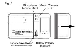
Carefully insert a fresh 9-volt alkaline battery, observing correct polarity as marked inside the battery compartment. The transmitter housing is designed to prevent incorrect installation of the battery. *Do not force the battery in.*
