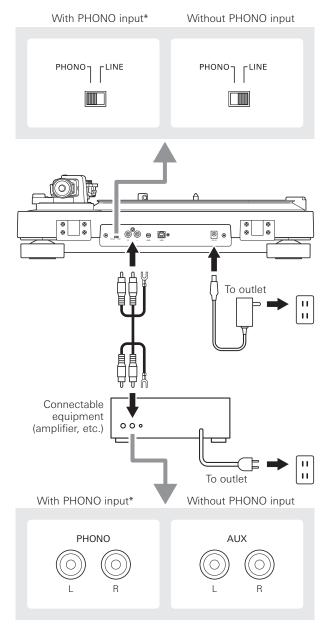
\* Depending on the equipment you are connecting, a ground (earth) terminal may exist near the phono input jack. If this is the case, connect to it using the ground line from the RCA audio cable. This will help prevent a low humming noise that might otherwise be heard during playback.
