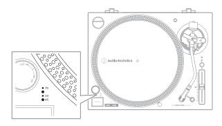
If the quartz button is pressed, the internal quartz lock will hold the platter at precise rated speed regardless of the position of the pitch adjust slide control.
