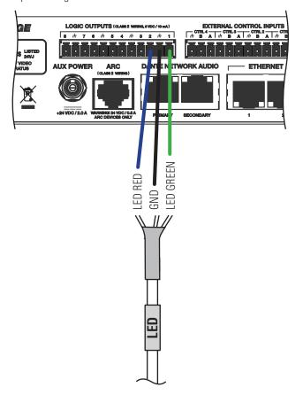
NOTE: The ES954 comes pre-terminated for use with the Audio-Technica ATDM-0604. When using the ES954 with Symetrix devices it *must be rewired as polarity is reversed.*
