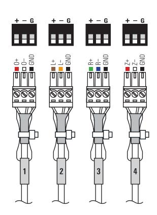
All QSC inputs and outputs use 3.5 mm Phoenix or euro-block connections.
