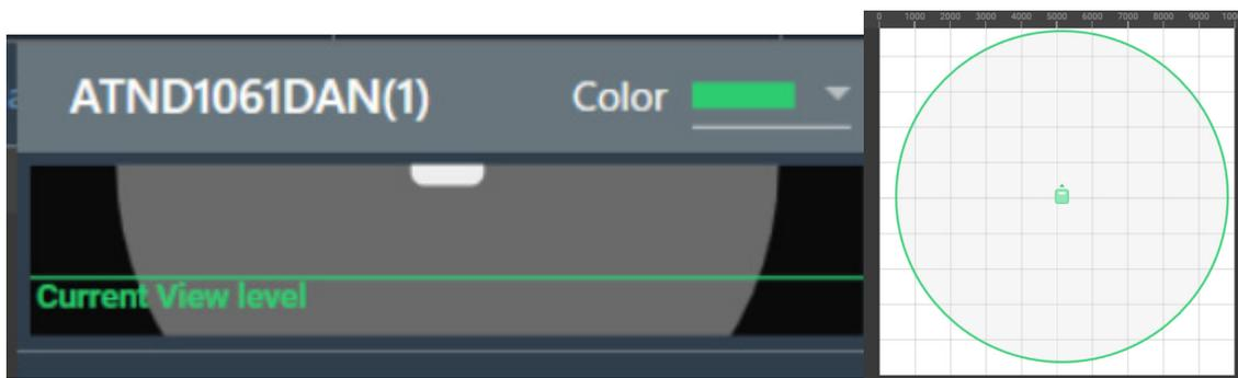
When the device is installed at a height of 2.6 m (8.5'), which is a typical ceiling height in offices, the talker detection range on a plane at a height of 1.1 m (3.6') is a circle with a radius of approximately 4.8 m (16').
