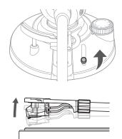
4. Position the tonearm over the desired location (groove) on the record.
