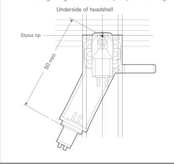
Mount the cartridge so it is perpendicular to the top of the headshell.
