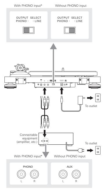
\* Depending on the equipment you are connecting, a ground (earth) terminal may exist near the phono input jack. If this is the case, connect to it using the ground line from the RCA audio cable. This may help prevent a low humming noise that might otherwise be heard during playback.
