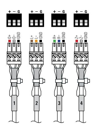
All Bose inputs and outputs use 3.81 mm Phoenix or euro-block connections.
