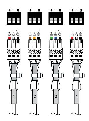
All Biamp inputs and outputs use 5.08 mm Phoenix or euro-block connections.
