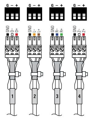
All Symetrix inputs and outputs use 3.81 mm Phoenix or euro-block connections.
