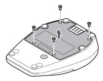
**2** Remove and replace the rechargeable battery.
