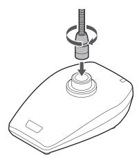
2 Use a hexagonal wrench to tighten the fixing screw, fixing the gooseneck microphone in place on the desk stand transmitter.
