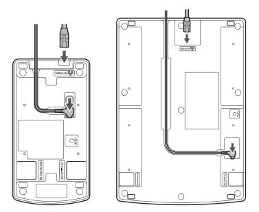
4 Insert the transmitters to use into the charging station.
