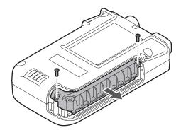
3 Remove and replace the rechargeable battery.
