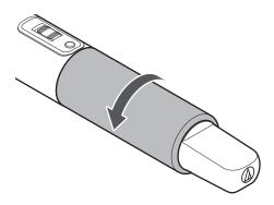
2 Remove and replace the rechargeable battery.
