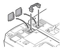
2 Attach the link plate with link plate screws.
