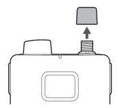
2 Connect the external microphone to the input connector and tighten the screw part.
