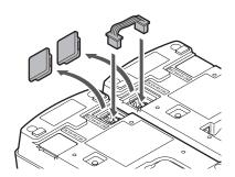
2 Attach the link plate with link plate screws.
