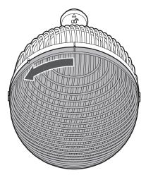
**2** Push the microphone module out from the inside of the windshield.
