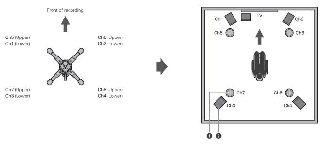
Speaker installed on the ceiling (upper section)
