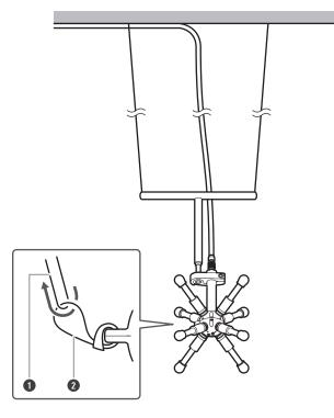
1 Seismic cable (not included)
