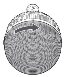
**4** Attach the microphone module to the core body.
