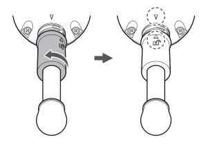
**2** Remove the microphone module.
