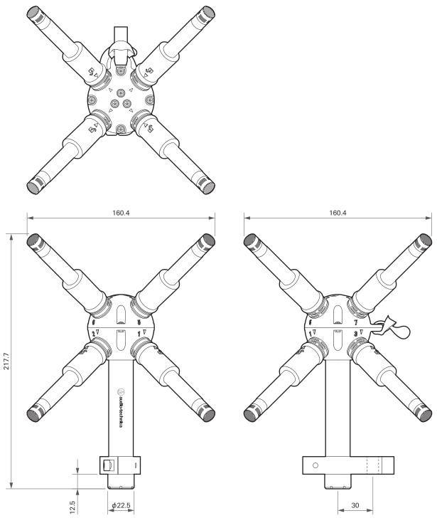
Distance from center of grip to center of screw hole
