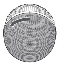
**2** Attach the bottom section of the windshield to the microphone module.
