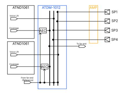
• Separate the signal systems for audio to be output from the speaker and the audio to be sent to the far end. Example: When using the ATDM-1012 or ATDM-0604a, this can be performed as shown below.
