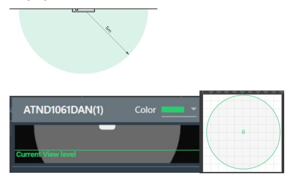
When the device is installed at a height of 2.6 m (8.5'), which is a typical ceiling height in offices, the talker detection range on a plane at a height of 1.1 m (3.6') is a circle with a radius of approximately 4.8 m (16').
