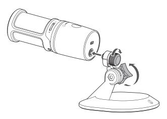
• Use the included 3/8"-16 to 5/8"-27 threaded adapter when installing the product on a commercially available microphone stand.
