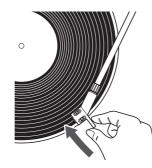
5 Lower the tonearm by moving the tonearm lift control lever to the DOWN position.
