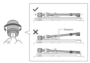
8 Set the tracking force gauge ring to the "0" position. After that, turn the counterweight and the tracking force gauge ring together counterclockwise (to the left) to the "2" position.
