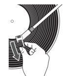
4 Lower the tonearm by moving the tonearm lift control lever to the DOWN position and fix it with the clamp.
