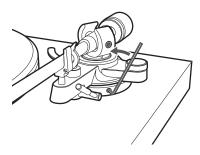
2 Adjust the tonearm height by manually lifting or lowering the tonearm assembly.
