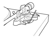
4 Place a record on the platter, position the cartridge over the record. Lower the stylus to the record surface, and confirm that the tonearm is parallel to the record's surface.
