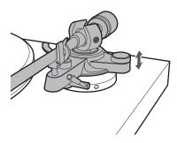
3 Reinsert the hexagonal wrench into the tonearm adjustment socket and turn it clockwise to lock the tonearm height.
