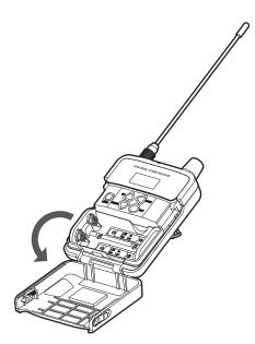
Insert the batteries according to the plus (+) and minus (-) marks found inside the battery compartment.
