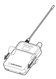
2 Open the battery cover while holding the latches down.
